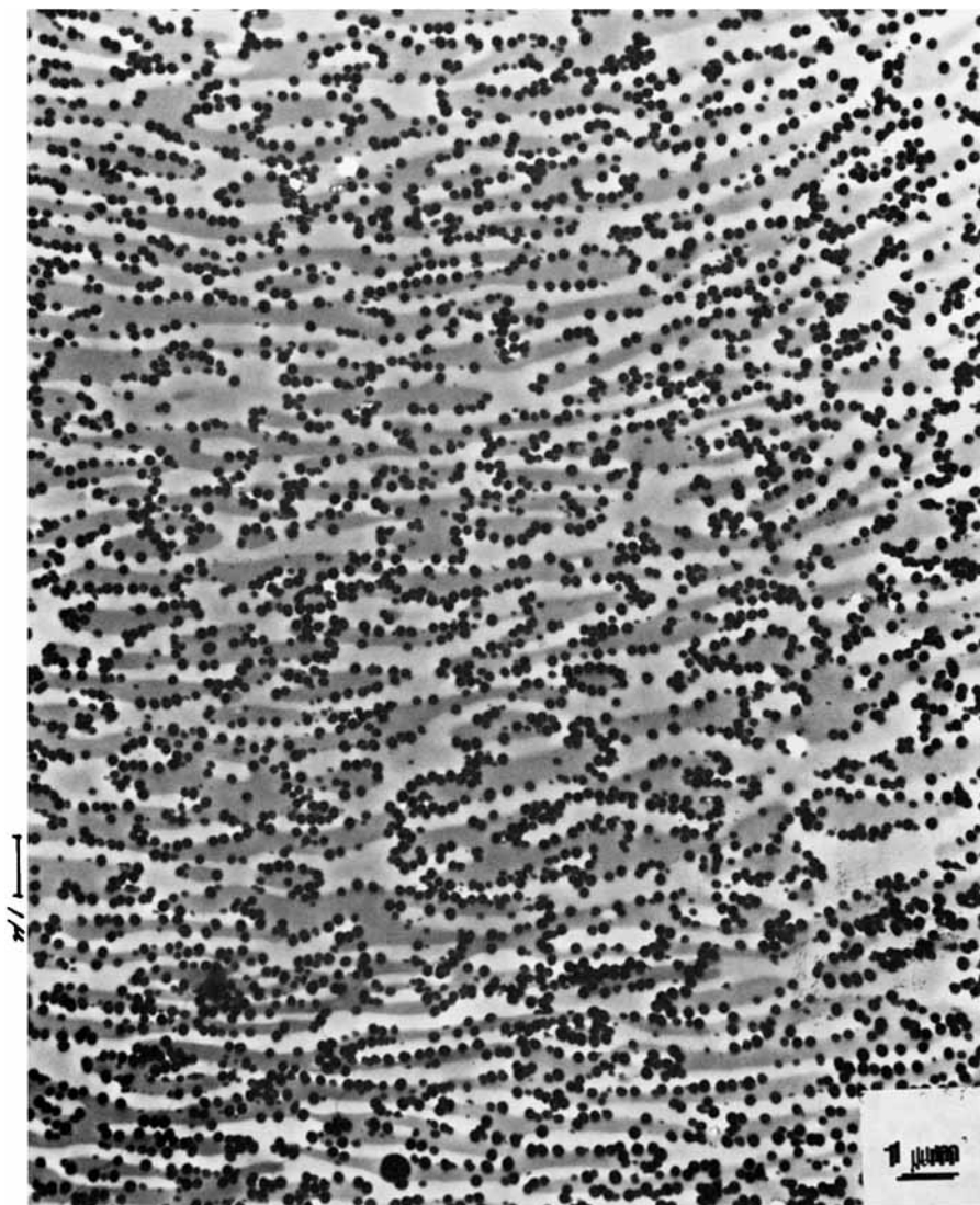
Fig. 3. Transmission electron photomicrograph of a PS/SAN/MBS (41/41/18) blend prepared by simultaneous mixing of the components in an extruder.
